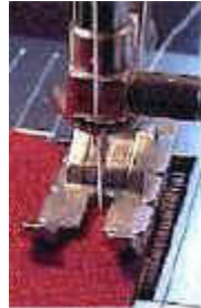
Quarter inch foot makes it easy to sew an accurate 1/4" seam
